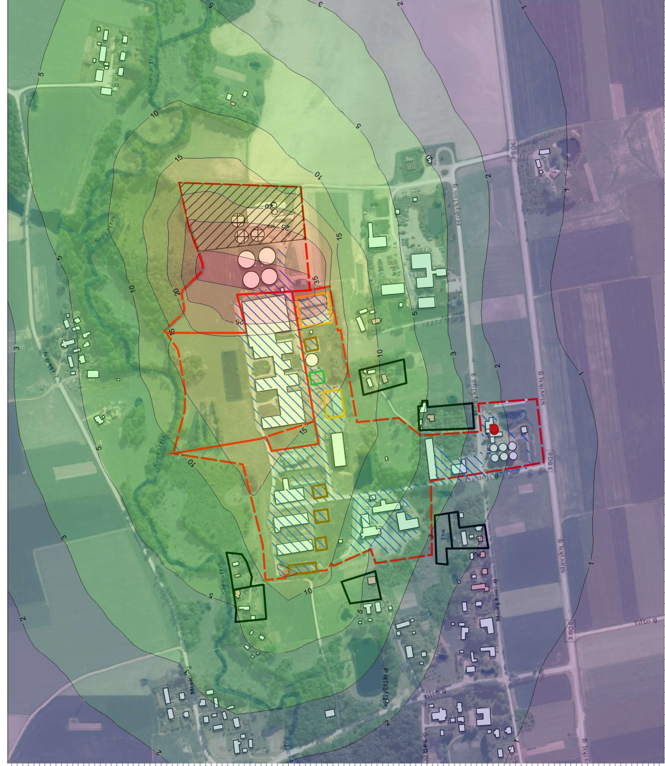
PLOT FILE OF 98,50TH PERCENTILE 1-HR VALUES FOR SOURCE GROUP: ALL Max: 39.9 [ug/m 3 ] at (428472.34, 6093036.04)
